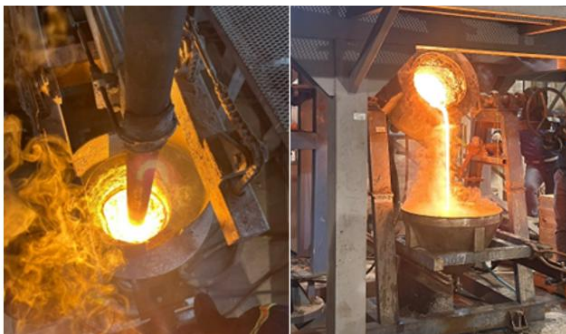
Figure 4. Reaction and casting in EAF.
