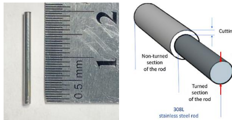
Figure 1. AISI 308L sample rod d=1.6 \text{ mm} , l=20 \text{ mm} and schematic representation of the turned and non-turned sections of the AISI 308L stainless steel rod.
