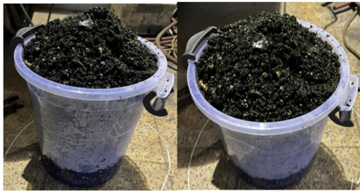
Figure 3. Metal slag mixed state of samples quenched in water TSII 6 and 7.
