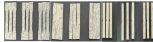
Figure 3. Composite specimens produced with 1%, 3%, and 5% fiber content
